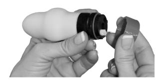
3. Remove the storage and safety cap from the Base Control Unit
