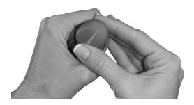
While applying slight pressure on the cap toward the attachment connector/motor housing, rotate the cap counter-clockwise. The cap will disengage from the attachment and can be completely removed.
