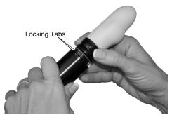
Gently slide the attachment down the motor shaft such that attachment seats down enough for the red O-ring to contact both the attachment connector/motor housing rim and attachment lip. You may need to wiggle the attachment slightly as the shaft slides up the inside of the attachment for it to seat completely.
