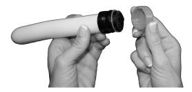
Notice the three locking tabs on the attachment that correspond to three slots on the storage cap. Align the tabs on the attachment with the slots on the cap and insert the attachment until the red O-ring is in contact with both the attachment lip seat and the safety cap rim.
