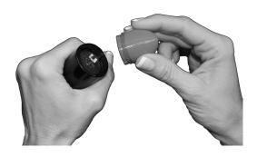
Notice that the safety and storage cap has three locking tabs that are guided by three corresponding slots on the attachment connector housing to insert the safety and storage cap.
