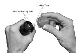
Gently slide the safety and storage cap into the slots such that safety and storage cap seats down enough for the red O-ring to contact the attachment connector housing.
